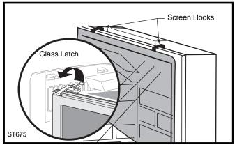
Fig. 35 Remove the screen or glass panel.
